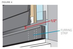
1/2" space between the siding and the flashing over all openings
